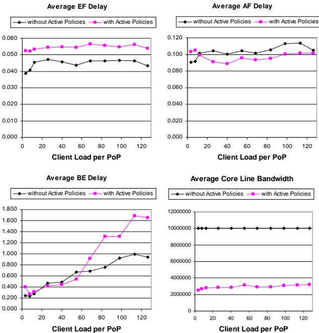
Fig. 7 Average delay and core bandwidth
