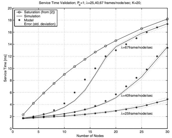
Figure 3. Average virtual service time  $T_S$  for different frame's rate generation.
