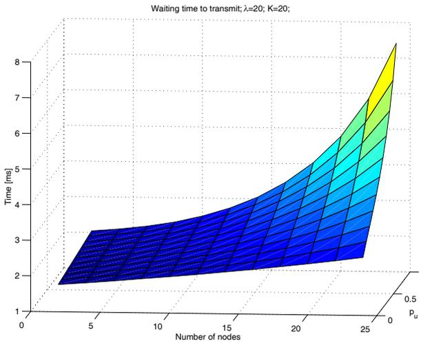
Figure 6. Model's numerical solutions for total delay.
