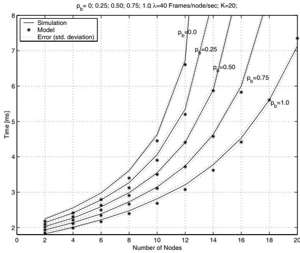
Figure 5. Total delay  $T_d$  considering different  $P_b$  values.
