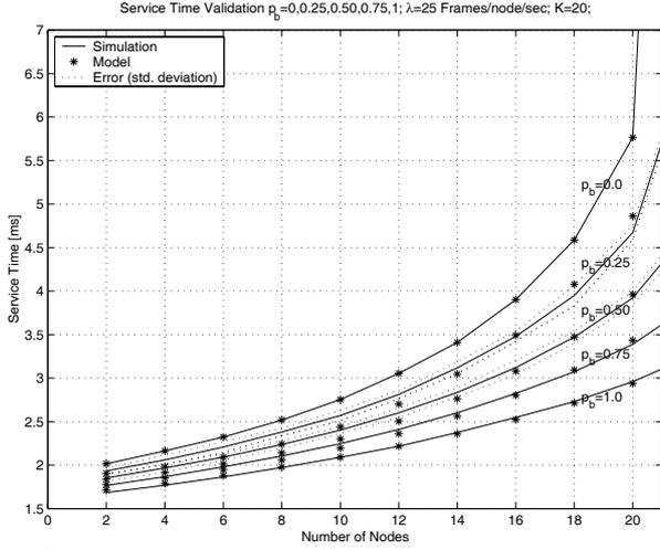
Figure 4. Average virtual service time  $T_s$  for different  $P_b$  values.
